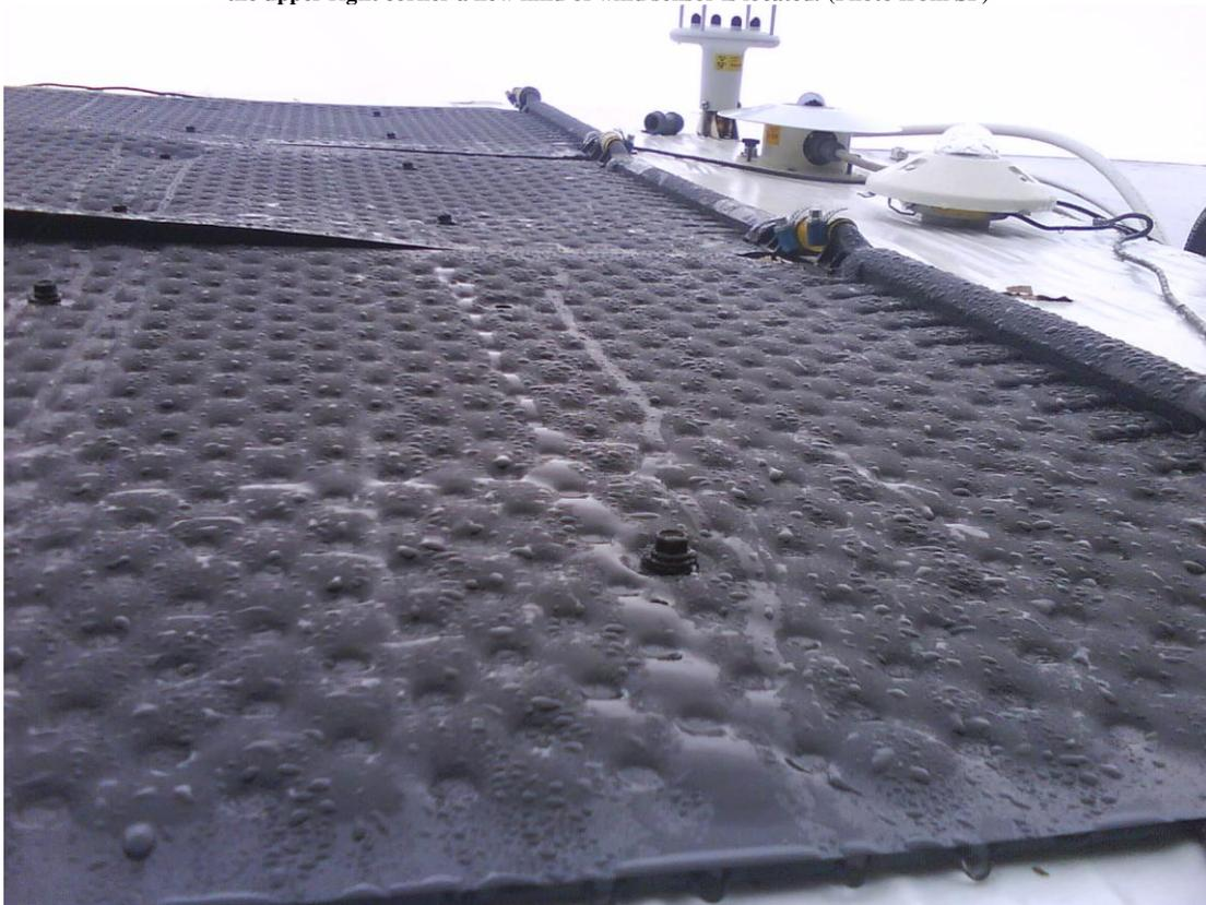
**Fig. 2: Close up of the collector absorber surface during condensation operation. A lot of water is “produced” so it is important to have a really water tight roof under the collector. Here the inactive round welding spots on the absorber can be seen too. This affects the parameter values somewhat from the ideal numbers. (Photo from SP)**
