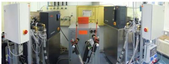
Fig. 5. Dynamic test facility for heat pumps at ITW
