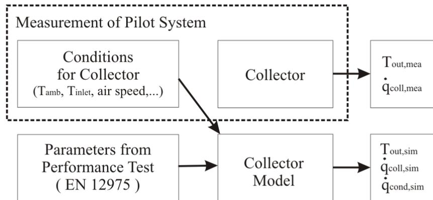
Fig. 2: Schematic procedure to determine the condensation gains in the monitored system from the measured data. The comparison of outlet temperature  $T_{out}$  and collector yield  $\dot{q}_{coll}$  indicates the accordance of simulation. The yield through condensation is determined within the simulation model.
