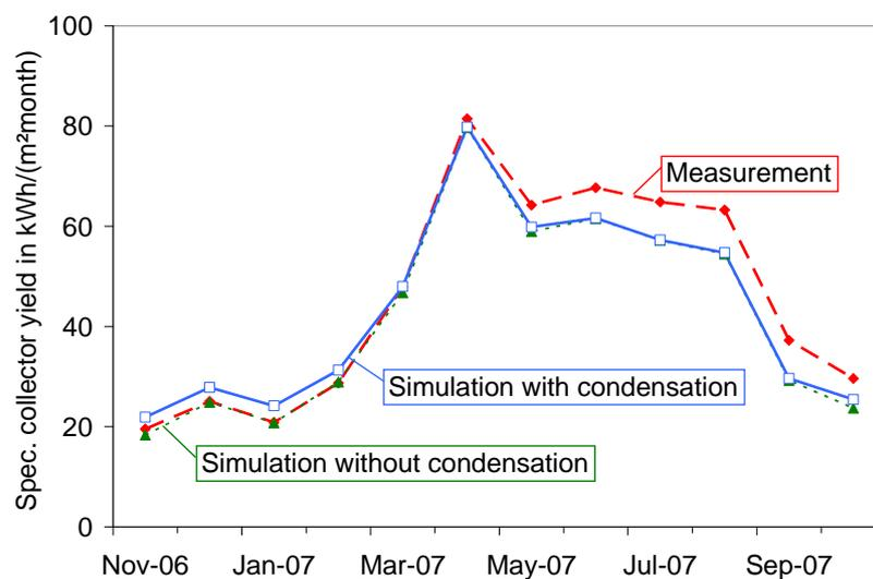
Fig. 4. Measured collector yield compared to simulations with or without condensation.
