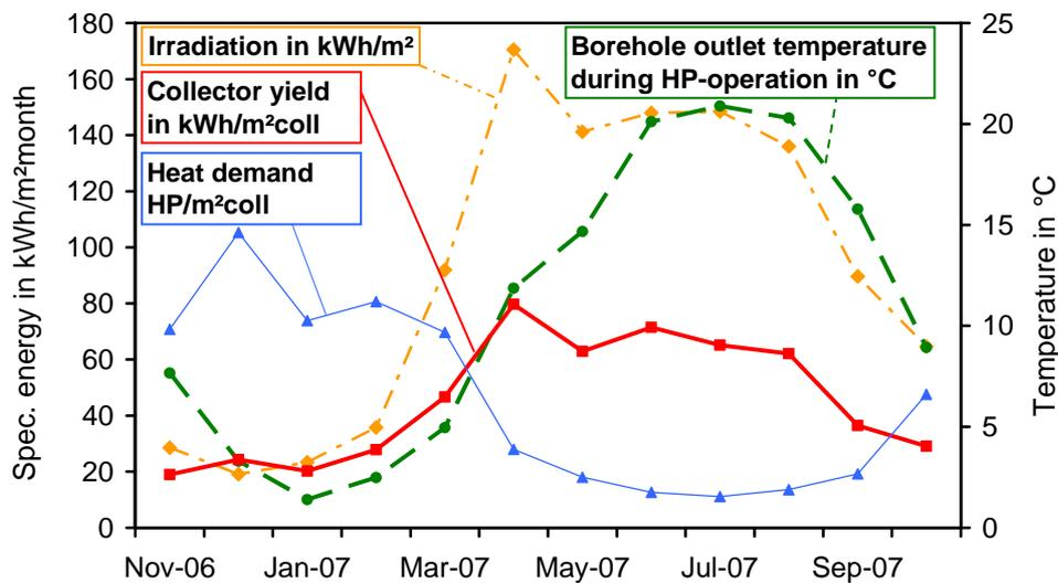
Fig. 2.: Measured monthly mean values of collector yield, heating demand at the heat pump evaporator, irradiation and borehole outlet temperature in the course of one year at the Limburg plant (Nov. 2006 - Nov. 2007)
