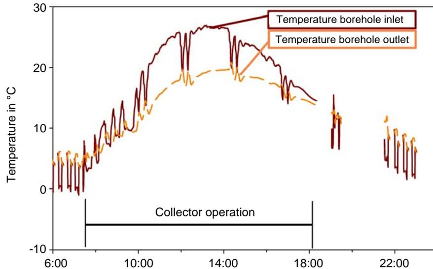
Fig. 3. Temperature at borehole in- and outlet in the course of day (8-Apr-2007, plant Limburg). The figure shows the temperatures while collector pump and HP are running.
