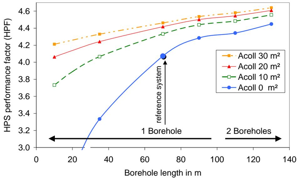
Fig. 5. Correlation of HPS performance factor (HPF), collector area and borehole length. Electric power consumption of the pumps is neglected.
