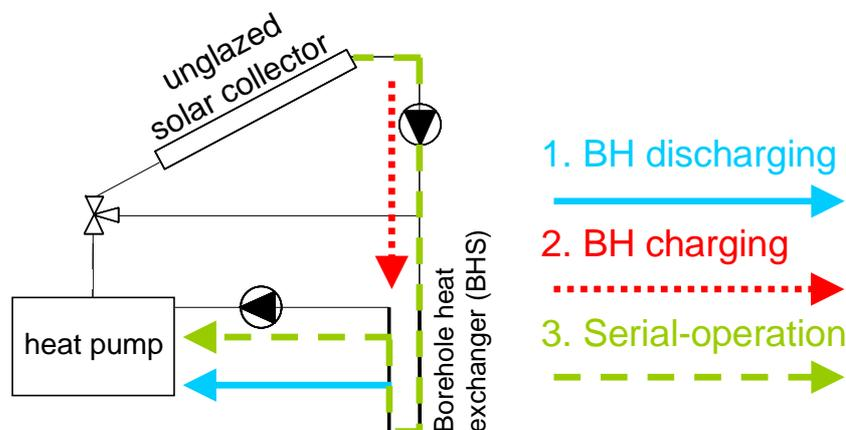
Fig. 1. System concept and operation modes. A common heat pump system with BHE is extended by an unglazed SC. Only the heat source side of the heat pump is shown.
