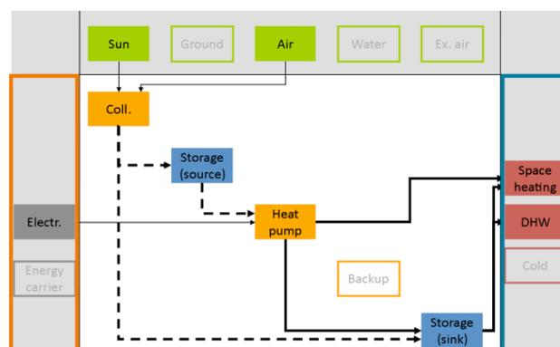
Using the square view to show one definition of the system performance (blue rectangle = the output divided by orange rectangle = the non local energy input)
