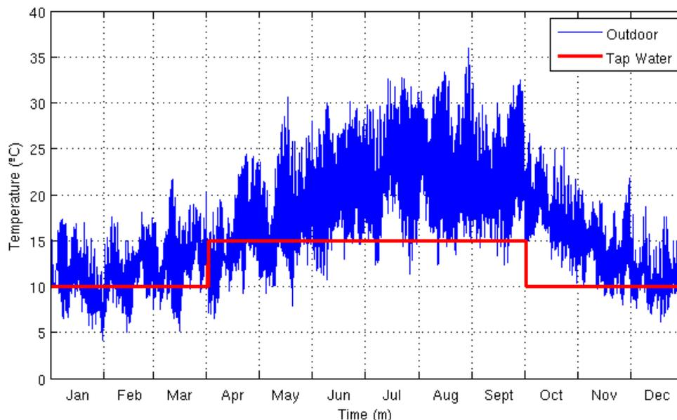
Fig. 4: Reference outdoor temperatures for the Lisbon municipality and assumed tap water temperatures
