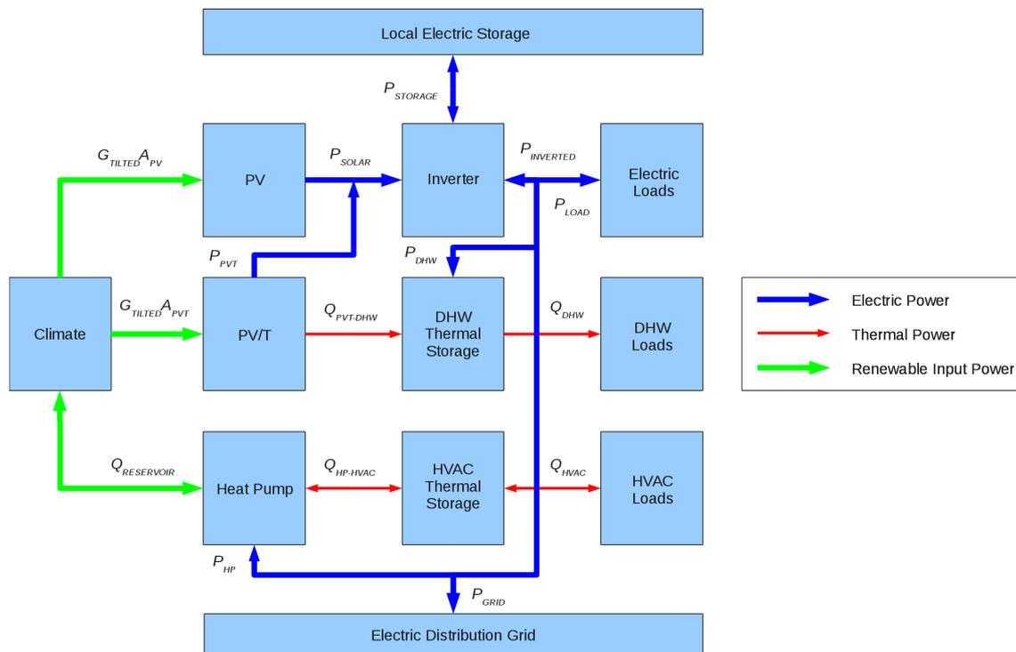
Fig. 3: Solar trigeneration system model power flow diagram
